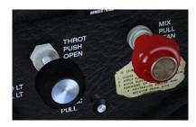
Figura 8.23: Throttle & mixture
