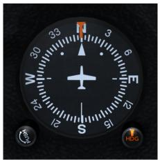
Figura 8.28: Magnetic compass & heading indicator
