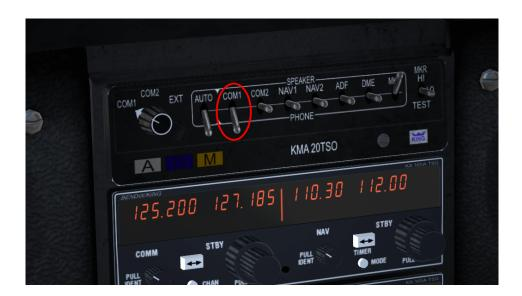
Figura 9.7: Speakers switch for COMM1
