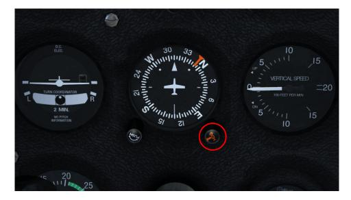
Figura 9.9: Heading adjust knob
