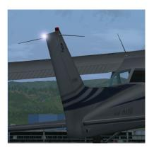
Figura 8.20: The tail rudder
