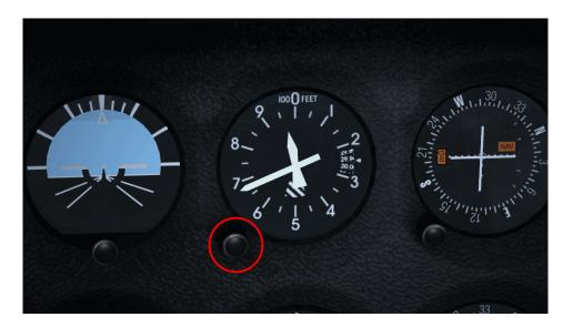
Figura 9.8: Altimeter calibration knob
