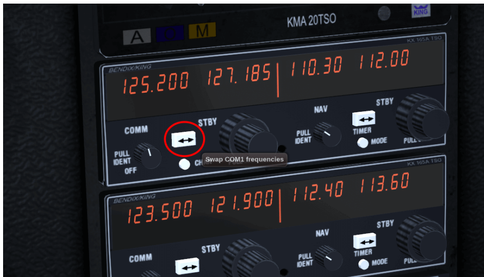
Figure 9.6: COMM1 transfer key to swap the frequencies
