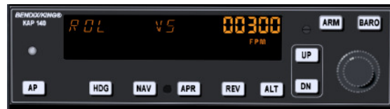
Figure 10.6: Autopilot after engaging
