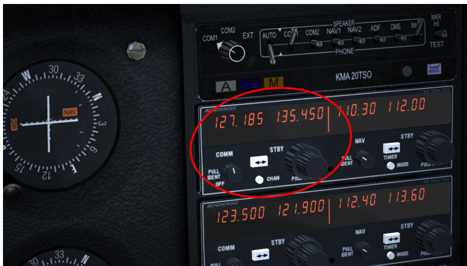
Figure 9.4: The C172 communications stack with COMM1 highlighted
