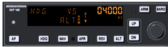
Figure 10.9: Autopilot with altitude armed
