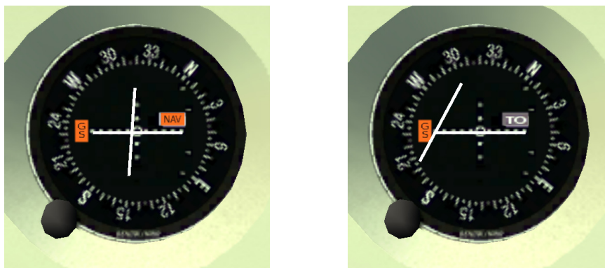
Figure 10.5: VOR1, before and after tuning
